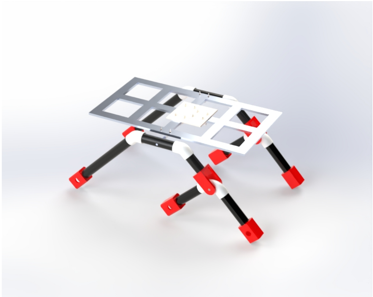
Figure 19: CAD Model of Rocker-Bogie Suspension
