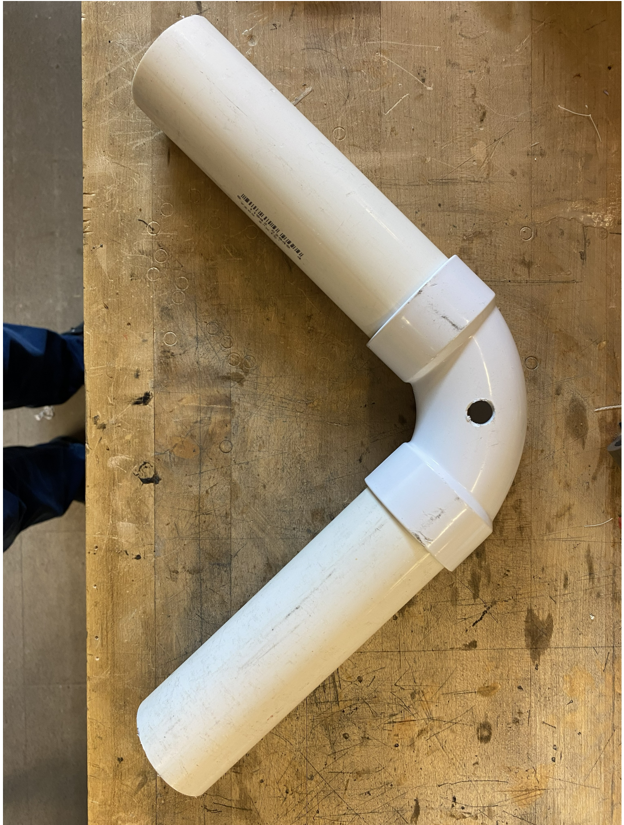
Figure 93: Bogie with Hole Drilled
