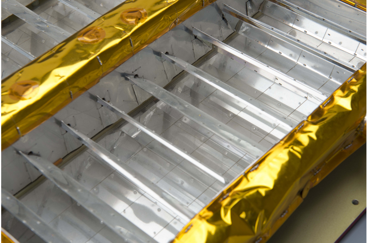
Figure 15: Rosetta Passive Thermal Louvers, European Space Agency
