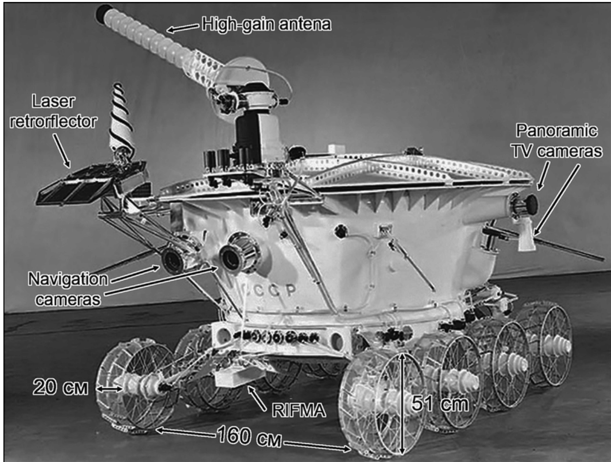
Figure 5: Image of Lunokhod 1 rover and navigation systems
