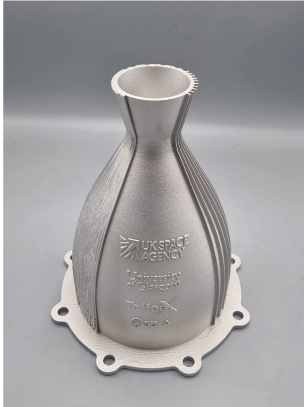
Fig. 17 Example of a 3D printed nozzle with optimized cooling channels
